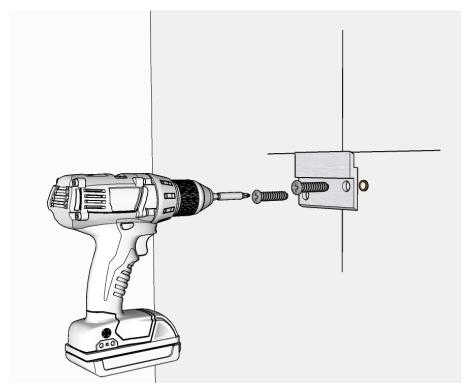
I. using #8 screws, secure french cleat to the wall
